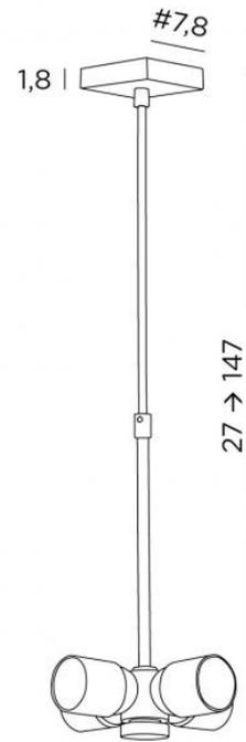
Suspension to place a lampshade (with special attachment in the lampshade). Including a square base, a set of adjustable tubes and a "Nourrice" with four E27 fittings. Adjustable in height when mounting
